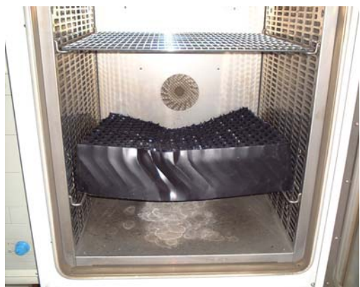
Deformation after 15 Minutes at 60°C
