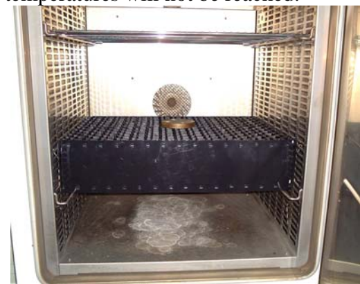
no deformation at 120°C after a total test length of 288 hours
